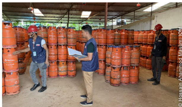
LPG cylinders were stored at the distribution point warehouse with adequate spacing between stacks prior to distribution. Vendor staff regularly inspected the cylinders to ensure safe storage.
