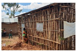
The main shelter typology in East Hararghe is typically a wooden structure that consists of wooden poles harvested locally, wooden infill from wild bushes, and mud plastered walls.
