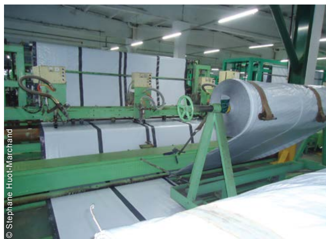
Suppliers started producing the new tarpaulin in the late 1990s. The use of reinforcement bands instead of eyelets allows for mechanization, increasing quality and speed of production.
