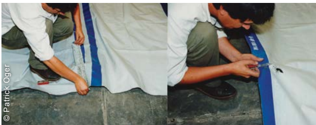
Peeling and scratching tests can be conducted in the field after basic training.
