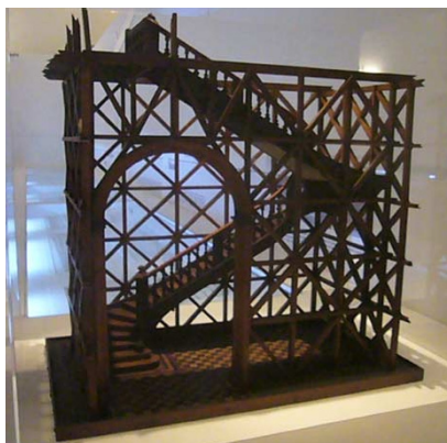
A model showing the Pombaline cage design. The design is said to have been tested by getting the army to walk up and down on the roof of a full-size model.
