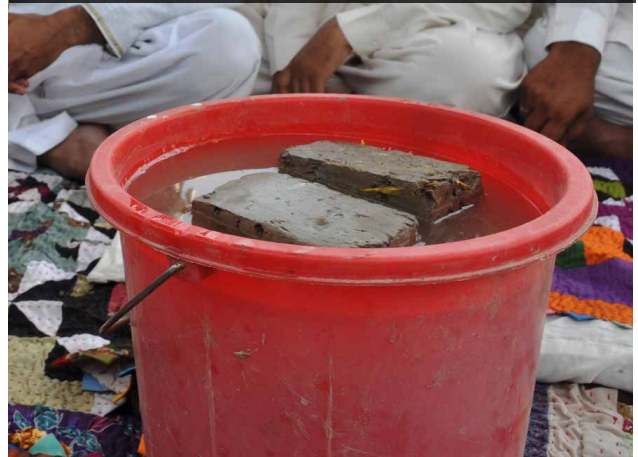
An important part of securing community confidence in new techniques: testing the durability of lime-stabilised soil blocks tunder water. These blocks had been in this bucket for about 6 months, so the community was confident that the materials would be flood-resistant. Photo: Magnus Wolfe Murray
